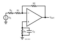
NOISE AT  $V_{OUT}$  IN  $V_{RMS} = V_{ON}$  IN  $V/\sqrt{Hz} \cdot \sqrt{f_{NBW}}$   $f_{NBW} = NOISE$  BANDWIDTH
