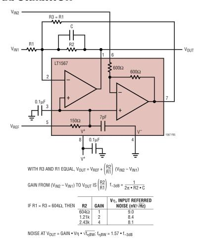
Figure 5. A Differential to Single Ended Amplifier/Filter
