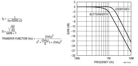
GAIN IS MEASURED TO EITHER OUTPUT ALONE. IF OUTPUT USED DIFFERENTIALLY,  $V_{OUT}^+ - V_{OUT}^- = 2 \times V_{IN}$
