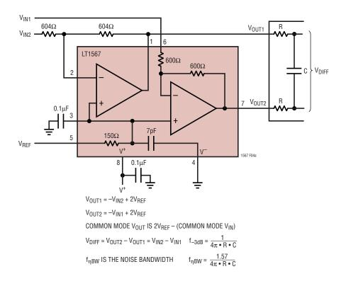
Figure 4. A Differential Buffer/Driver
