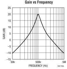
GAIN IS MEASURED TO EITHER OUTPUT ALONE. IF OUTPUT USED DIFFERENTIALLY,  $V_{OUT}^+ - V_{OUT}^- = 2 \times V_{IN}$
