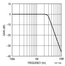
GAIN IS MEASURED TO EITHER OUTPUT ALONE. IF OUTPUT USED DIFFERENTIALLY,  $V_{OUT}^+ - V_{OUT}^- = 2 \times V_{IN}$
