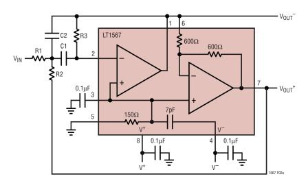
DESIGN EQUATIONS FOR  $f_{CENTER} \le 1MHz$   $f_{CENTER}$  IS THE FILTER'S CENTER FREQUENCY
