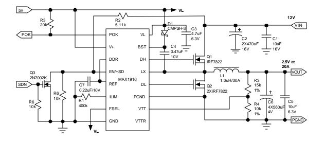
This circuit has been tested in the lab. The efficiency is about 88.5% at 20A output current. It should be noted that the prototype of this circuit is modified from the 7A VTT EV kit. The copper is only 1 Oz and the bottom two MOSFETs are stacked on top of each other due to single MOSFET layout. For a better layout, the efficiency will be better.
