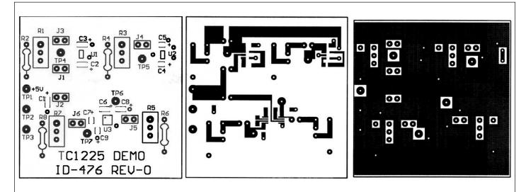
Figure 4. TC1225 DEMO Card Assembly Drawing and Artwork
