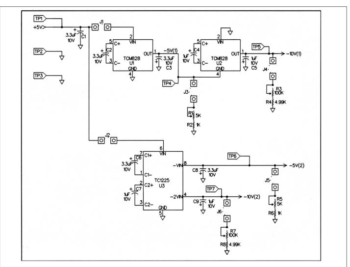
Figure 3. TC1225 DEMO Card Schematic
