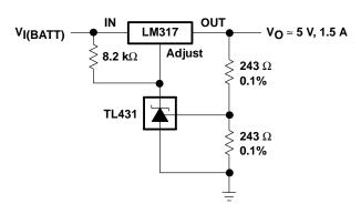
Figure 23. Precision 5-V 1.5-A Regulator
