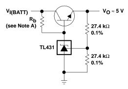
NOTE A:  $R_b$  should provide cathode current  $\geq 1$  mA to the TL431.
