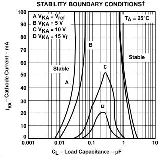
$<sup>\</sup>dagger$  The areas under the curves represent conditions that may cause the device to oscillate. For curves B, C, and D, R2 and V+ were adjusted to establish the initial V<sub>KA</sub> and I<sub>KA</sub> conditions with C<sub>L</sub> = 0. V<sub>BATT</sub> and C<sub>L</sub> then were adjusted to determine the ranges of stability.
