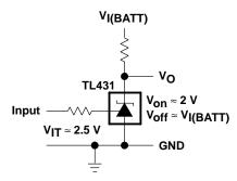
Figure 18. Single-Supply Comparator With Temperature-Compensated Threshold
