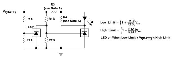
NOTE A: R3 and R4 are selected to provide the desired LED intensity and cathode current ≥1 mA to the TL431 at the available V<sub>I(BATT)</sub>.
