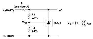
NOTE A: R should provide cathode current ≥1 mA to the TL431 at minimum V<sub>I(BATT)</sub>.
