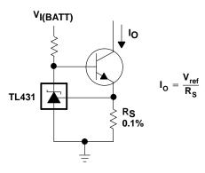
Figure 29. Precision Constant-Current Sink
