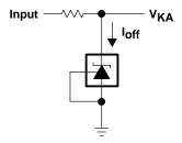
Figure 4. Test Circuit for Ioff
