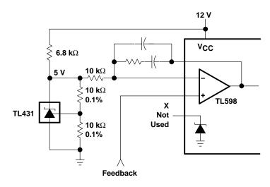
Figure 25. PWM Converter With Reference
