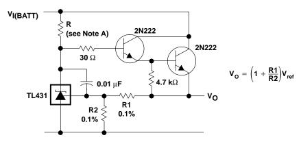
NOTE A: R should provide cathode current ≥1 mA to the TL431 at minimum V<sub>I(BATT)</sub>.
