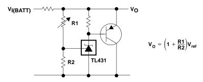
Figure 21. High-Current Shunt Regulator
