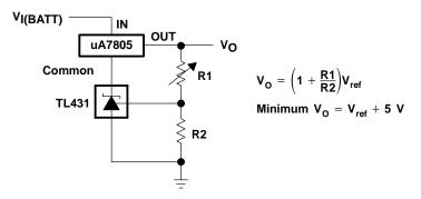
Figure 20. Output Control of a Three-Terminal Fixed Regulator
